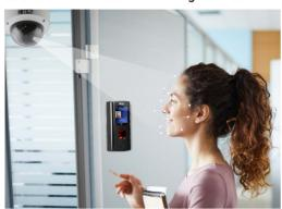
Matrix COSEC Device based (COGNIFACE) Facial Recognition is a unique solution with IP Camera and COSEC door controller to offer very accurate user identification even in challenging working conditions for time-attendance and access control applications.
